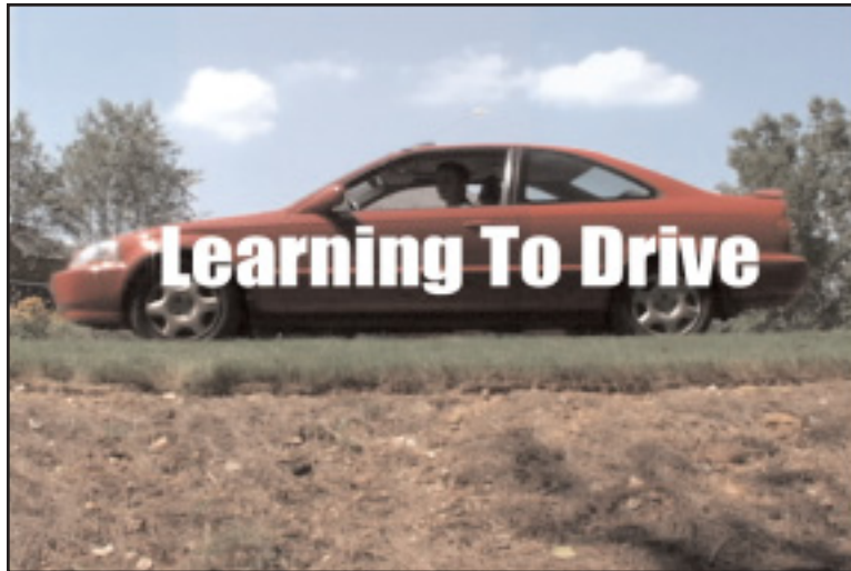
Figure 6.16 DV image and title at 720 x 480 on a computer monitor. The title was made at 720 x 540 and compressed down.
