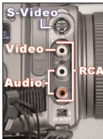
Figure E.8 RCA and S-Video ports on a video camera.
