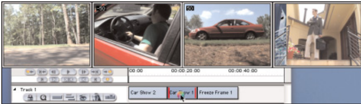
Figure 4.34 When you perform a a slip edit, Trim Edit Windows show you the first and last frame of the clip being adjusted. No other clips are affected.
