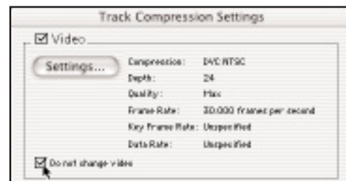
Figure 8.4 Clicking the 'Do Not Change...' check-box for Audio and Video means that the media type will render out unchanged.
