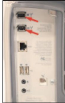
Figure E.2 The FireWire ports on a PowerMac G4 tower.
